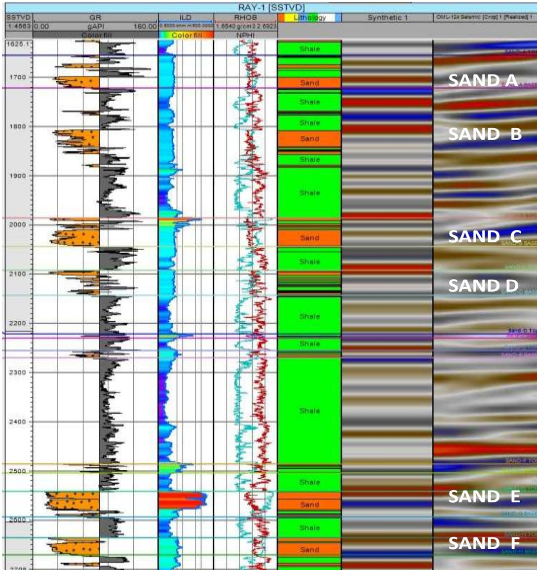
Fig. 3: Studied reservoir sand intervals along Well RAY-1 Well
